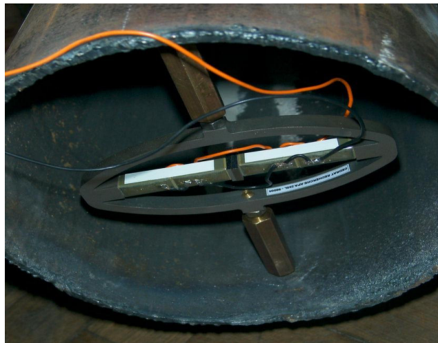
Fig. 8. The APA 230L activator (cf. [5]) inside the tube.
